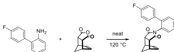
Figure 4.5 Synthesis of rotor (Ph-F)
